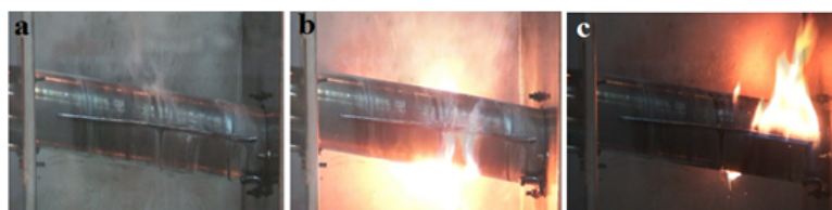
Fig. 4. Rapeseed oil tested on the manifold having a temperature of 530 \pm 5^\circ\text{C} : a. 1 st s; b. 2 nd s; c. 9 th s
