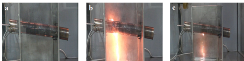
Fig. 6. The olive oil, tested at a manifold temperature of 500°C: a. 1 st s; b. 2 nd s; c. 23 rd s
